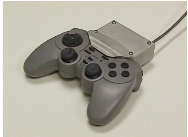
Figure 7. Videogame controller. We use a retrofitted off-the-shelf video game controller for high level control of gaze, movement and emotion. The well-designed physical interface allows the operator to quickly master the capabilities of the robot.
