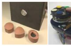
Figure 3: Tagged Handles. Detachable physical knobs with distinctive shape can be connected to a single haptic device (left). A functional prototype with top-mounted textural tags aids in switching functions, by pressing different tags.
